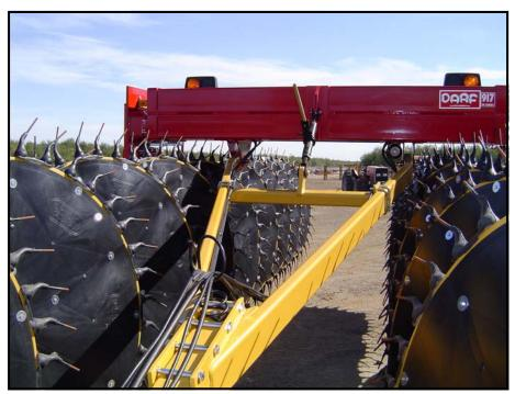
RUN POWER LEADS DOWN TONGUE WITH HYDRAULIC HOSES AND THROUGH HOSE HOLDERS TO FRONT OF RAKE. EXCESS CABLE LENGTH CAN BE TRIMMED AND CONNECTORS RE-ATTACHED FOR A CUSTOM FIT.
