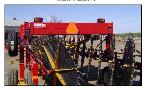
INSTALL MAGNETIC MOUNT LIGHT UNITS ON TOP FRAME AS SHOWN, ROUTE POWER CABLES THROUGH FRAME DOWN TO UPPER TONGUE
