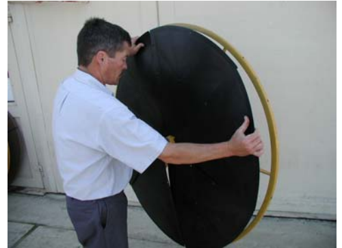
OVERLAP PIE SHAPED SECTIONS TO FORM FLAT JOINT
