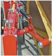
DARF's heavy duty trailing mounted cranks make for the gentlest hay handling. With the proper pitch and spring tension, the 52" wheels gently lift and turn the hay.
