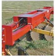
Twin sliding frame stabilizes the DARF Rake in rough fields. Fully open frame allows for 22' raking widths on the 950, 24' on the 917 and 29' on the 917W models.
