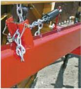
Rake wheel height adjustment is quick and easy with the DARF spring linkage assembly. Dual slots allow for chain adjustment to be positive, precise and fast.
