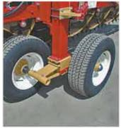
Heavy duty walking beams allow for fast, smooth field operation and easy road transport.
