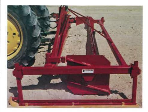
Note the Long Sled Runners which provide excellent flotation even on loose ground. You can increase or decrease the size of the border by the amount of dirt you carry; this is controlled by the up & down adjustment of the runners.
