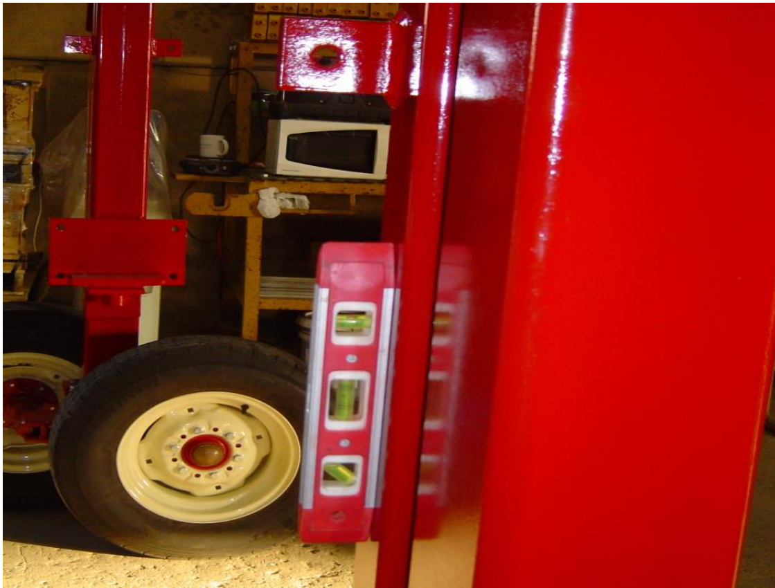
Square, level, and securely tighten the junction of the leg struts with the overhead main frame
