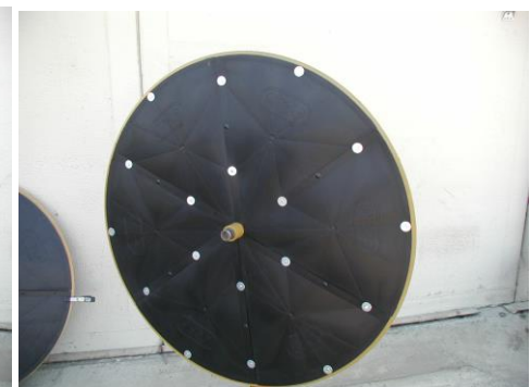
FASTEN TO RAKE WHEEL USING STD. FASTENERS IN TOP & BOTTOM HOLES ON JOINT. FASTEN OUTSIDE EDGES USING (1) SHORT FASTENER, (2) FLAT WASHERS, AND (1) NUT.
