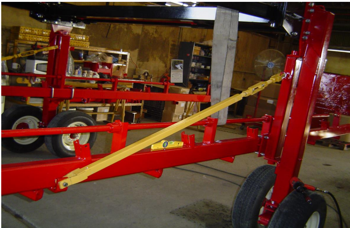
Adjust the front brace (9099) until the raking frame is square with the leg struts, then tighten the U-Bolts securely. **DO NOT TIGHTEN THE U-BOLTS UNTIL THE UNIT IS COMPLETELY LEVEL!! At this point you may tighten all nuts and bolts previously “snugged”
