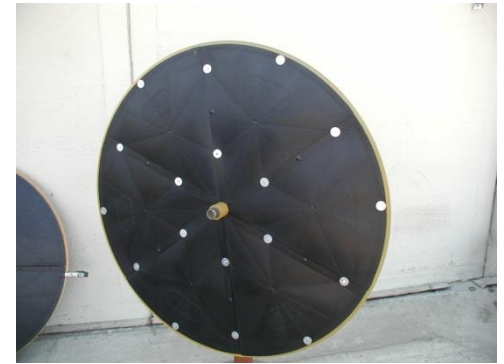
FASTEN TO RAKE WHEEL USING STD. FASTENERS IN TOP AND BOTTOM HOLES ON JOINT. FASTEN OUTSIDE EDGES USING (1) SHORT FASTENER, (2) FLAT WASHERS, AND (1) NUT.
